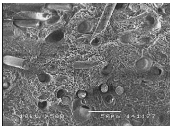
Figure 3 Poor fiber-matrix interface in N8G2.
